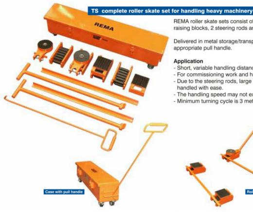
REMA roller skate sets consist of 4 rollers, 2 bogies, 2 raising blocks, 2 steering rods and 2 connecting rods.
